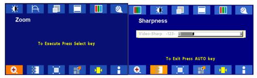
Push the select button Use "Left" or "Right" button to adjust Push the select button Use "Left" or "Right" button to adjust
